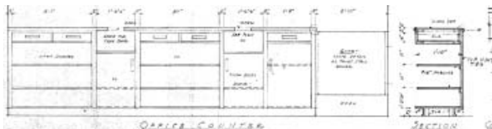
DETAIL OF COUNTER BETWEEN GENERAL OFFICE AND PUBLIC AREA FROM PERSPECTIVE OF OFFICE. UNDATED DRAWING COURTESY OF THE WASHINGTON MILITARY DEPARTMENT.
